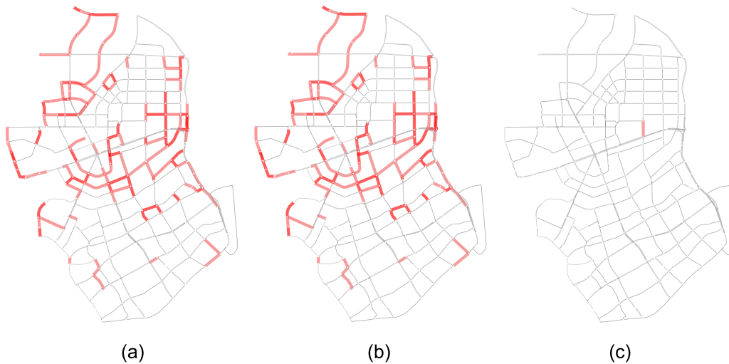
FIG. 9. Detection of the bottlenecks. The removed edges are indicated by thick red lines, and the remaining edges are indicated by thin gray lines, where the shades of red vary, with darker color indicating that the edges are broken in both directions and lighter color indicating only one direction is broken. (a) Removed edges before the critical point. (b) Removed edges at the critical point. (c) Bottleneck: Zhongyuan Road from south to north.
